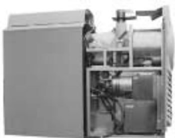
In 2000 Chugach and AVEC received and installed a 29-kw, gas-fired microturbine and began testing it at AVEC headquarters. An oil-fired unit arrived late in the year.
